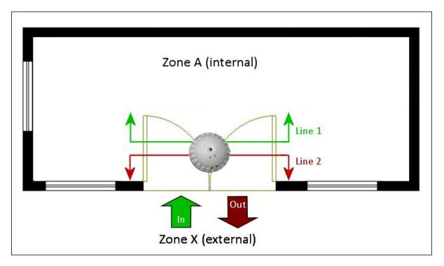
In order to represent this scenario we will need to program the Irisys IP counter with the correct IDs for each line. To do this we will allocate a 2-character ID to the entrance. Both lines belong to the same entrance, as one counts the *In* direction and the other the *Out* direction.
